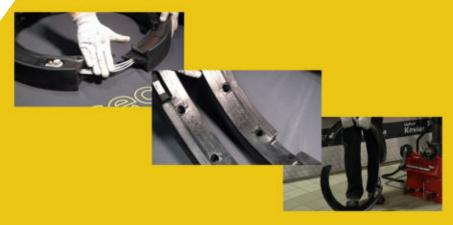
Check that cables are properly secured and make lock nut turn one click per size. Apply WD40 to locking nut or spring if necessary.
